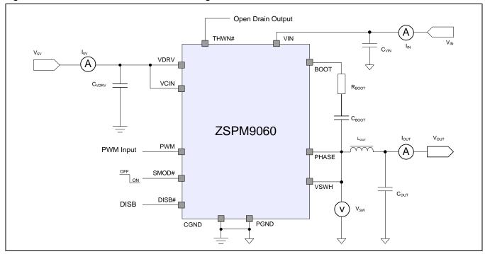
Figure 3.2 Power Loss Measurement Block Diagram
