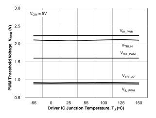
Figure 1.15 SMOD# Thresholds vs. Temperature
