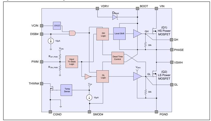
Figure 2.2 ZSPM9060 Block Diagram
