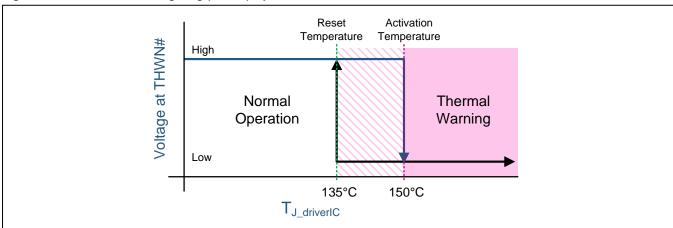
Figure 2.3 Thermal Warning Flag (THWN) Operation
